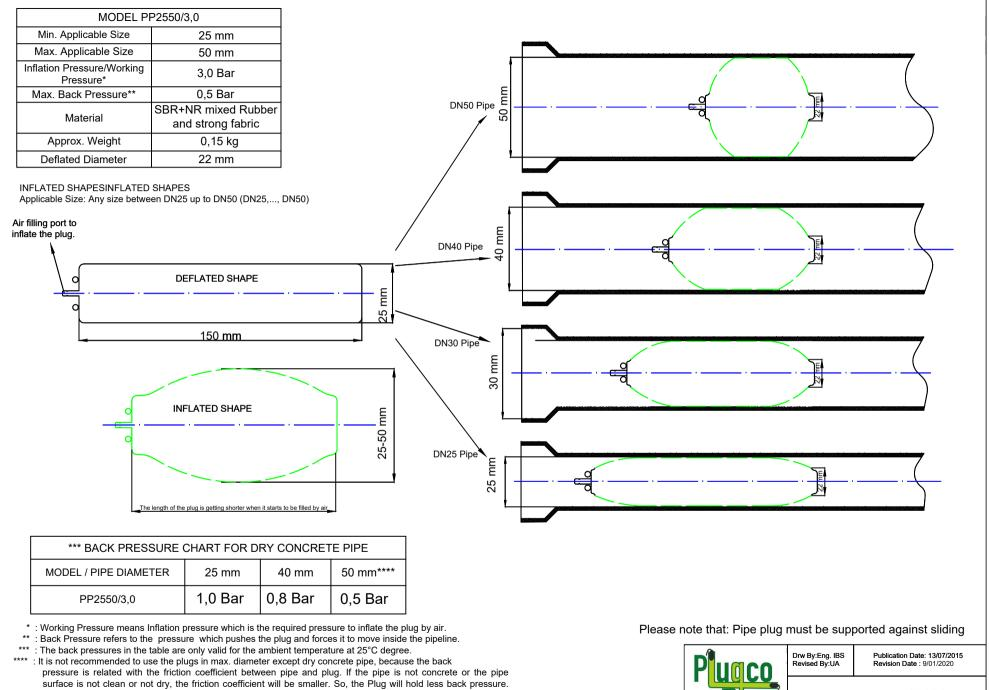
So, don't use the plug in limits and select the larger size plug for that kind of applications.
